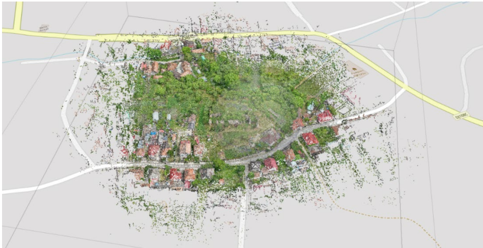
Fig. 5. Georeferenced point cloud of Bocskai Castle generated from the UAV photogrammetric dataset.
