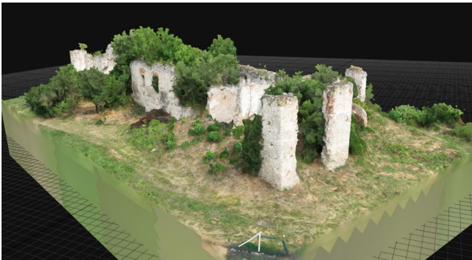
Fig. 8. Final textured three-dimensional representation of Bocskai Castle derived from UAV photogrammetry
