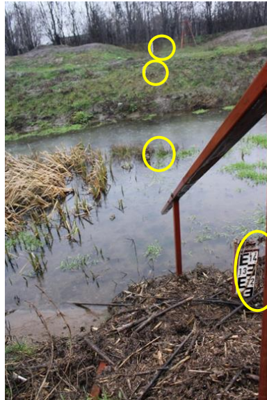
Fig.3. Hydrometric grom located on the river Suhu, at the Pechea hydrometric station (8.01.2021)
