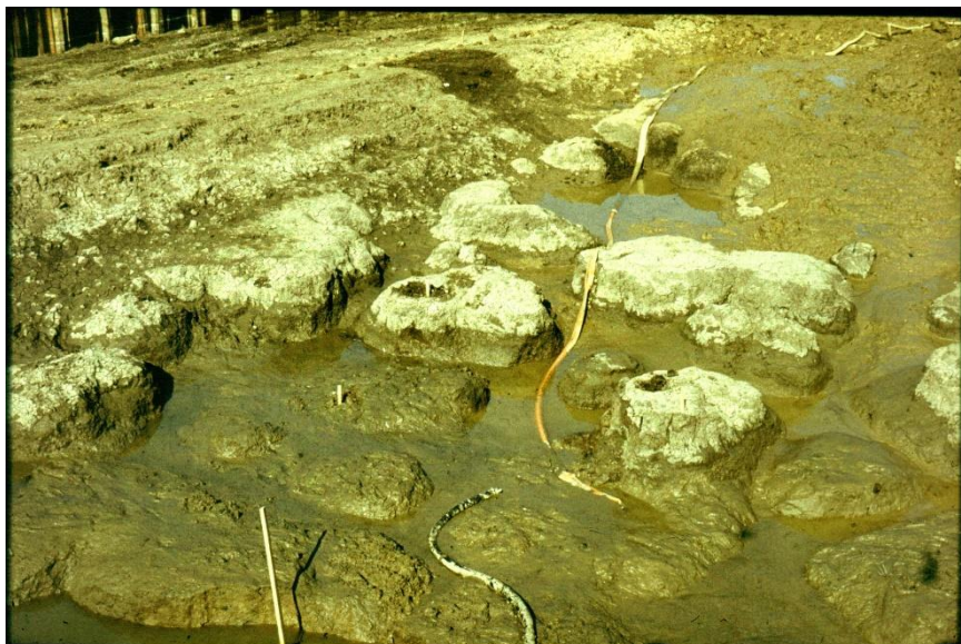
Figure 1. Dispersive soil after the flood in 1980
